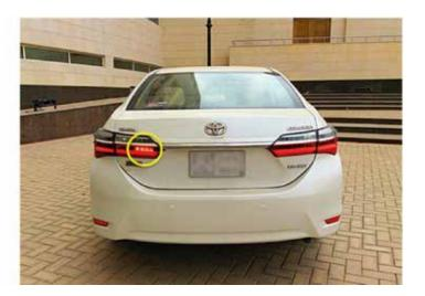
Taillights with rear fog light Rear fog lights should only be used when there is fog, snow, or heavy rain.
