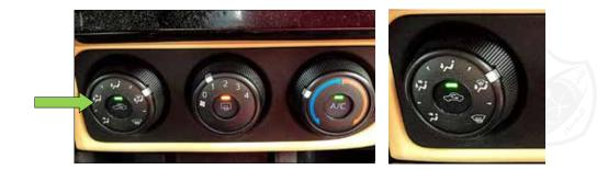
**Central key:** Air circulation inside the vehicle (e.g. when driving in tunnels.)
